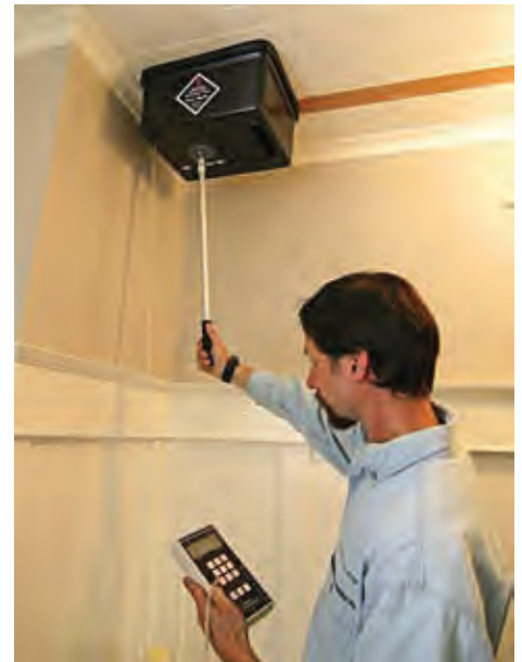
An exhaust fan flow meter helps accurately determine how well exhaust fans are operating.
