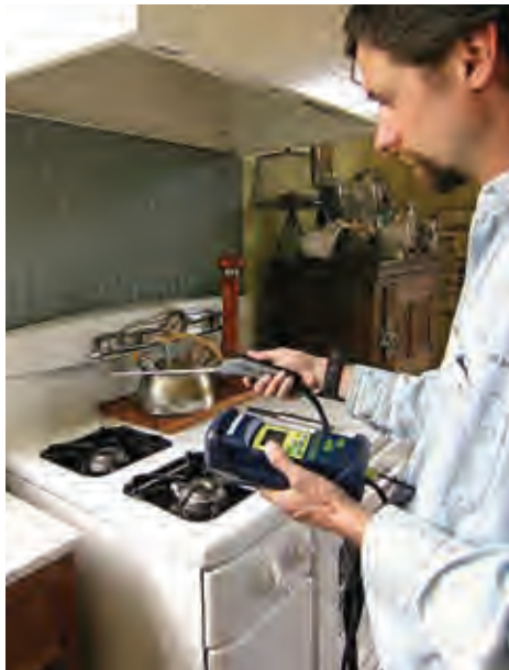
The carbon monoxide output of this vintage gas range is being checked.
